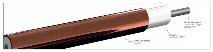
Low-loss semi-rigid cables provide lower attenuation, better phase stability with temperature, and a higher operating temperature compared to traditional solid PTFE semi-rigid cables.
