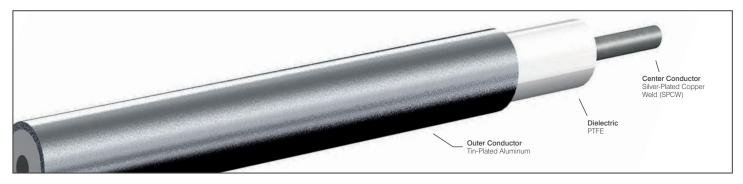
Our 50 Ω aluminum semi-rigid cables are ideal for hand forming or where weight savings is a premium. Connectors can be easily soldered to the tin-plated aluminum outer conductor.
