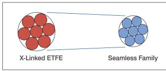
Example: A wire bundle of ten 20 AWG composite wires can be routed in the area required by eight XL-ETFE wires.
