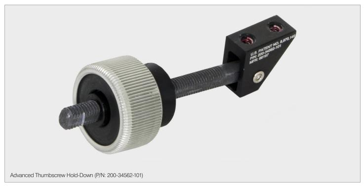
CarlisleIT's Advanced Thumbscrew Hold-Downs are the lightweight, high-performance option for when a more advanced hold-down solution is needed. Developed to meet the extreme performance standards of ABS1699, ASNA2168, and RTCA/DO-160, these hold-downs retain equipment even when not fully tightened and provide superior installation force compared to standard military-style hold-downs.
