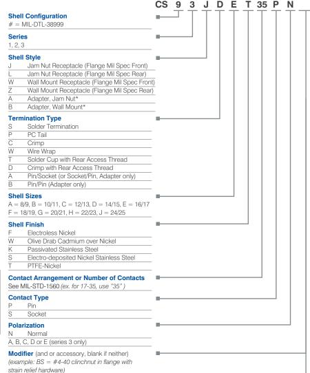
\*Note: All adapters are double receptacle, pin/skt, skt/pin, or pin/pin. Due to pattern symmetry, not all MIL 1560 patterns are available. Contact-type pin or socket denotes the front side of adapter connectors. For all other adapter requirements, contact us for PN assistance.
