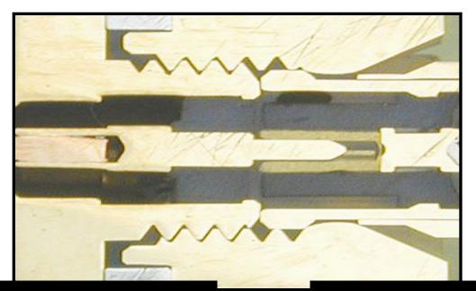
Pin shoulder could damage fingers
