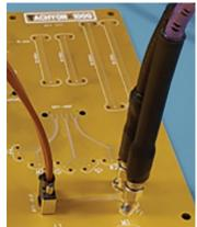
Fig. 13: CoreHC interconnect on a CPW PCB cross section
