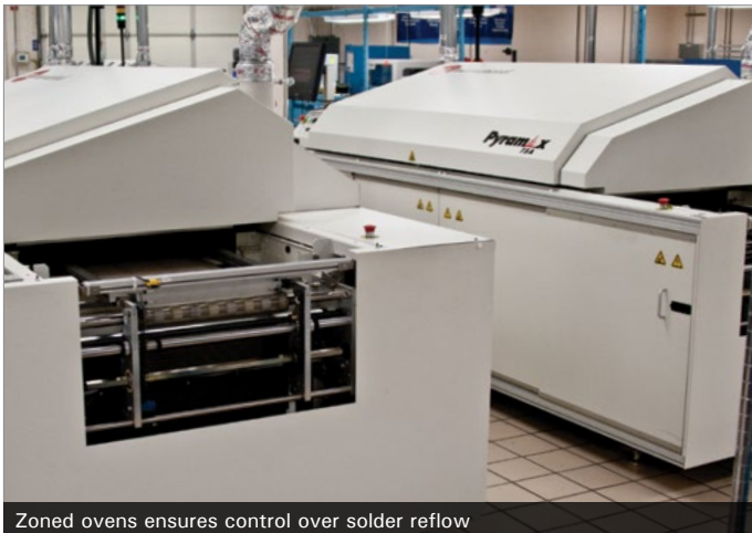
Zoned ovens ensures control over solder reflow
