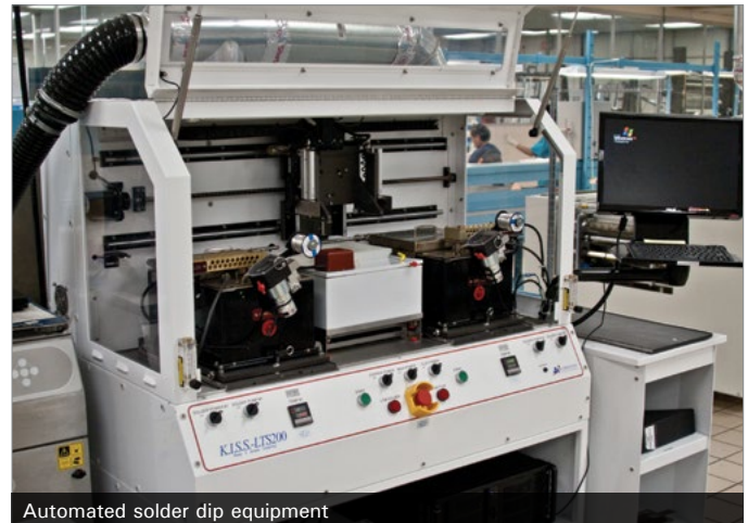
Automated solder dip equipment
