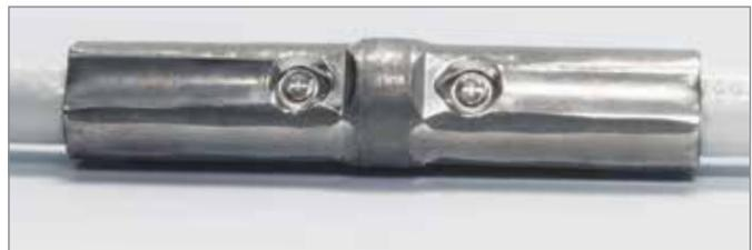
**Crimp Indicators:** Crimp indicators are embossed during the crimping operation, providing a visual indication of full wire insertion and proper connector installation.
