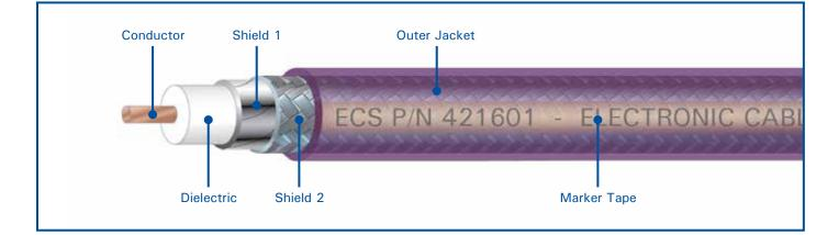
Conductor: 16 AWG solid copper wire Dielectric: High temperature fluoropolymer Shield 1: Aluminum tape Shield 2: Tin-plated copper braid Jacket: Purple high temperature fluoropolymer
