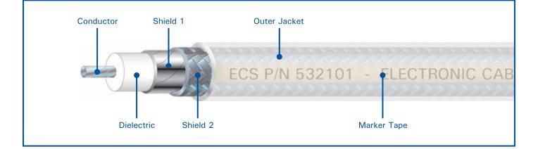
Conductor: 22 AWG stranded silver-plated copper Dielectric: High temperature fluoropolymer Shield 1: Aluminum tape Shield 2: Tin-coated copper braid Jacket: White high temperature fluoropolymer (laser markable)
