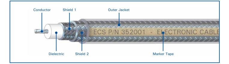
**Conductor:** 20 AWG stranded silver-plated copper **Dielectric:** High temperature fluoropolymer **Shield 1:** Silver-plated copper braid **Shield 2:** 38 AWG silver-plated copper braid **Jacket:** Clear high temperature fluoropolymer
