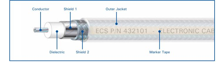
Conductor: 20 AWG stranded silver-plated copper Dielectric: High temperature fluoropolymer Shield 1: Aluminum tape Shield 2: Tin-plated copper braid Jacket: White high temperature fluoropolymer (laser markable)
