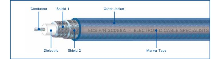
**Conductor:** 20 AWG silver-plated copper **Dielectric:** High temperature fluoropolymer **Shield 1:** 36 AWG tin-plated copper braid **Shield 2:** 36 AWG tin-plated copper braid **Jacket:** Blue high temperature fluoropolymer
