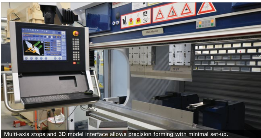
Multi-axis stops and 3D model interface allows precision forming with minimal set-up.
