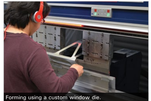
Forming using a custom window die.
