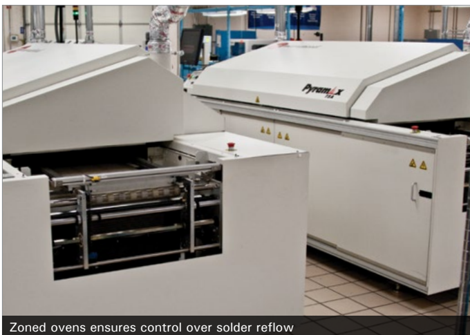
Zoned ovens ensures control over solder reflow
