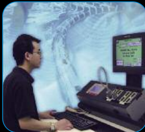
Cirris 1500V Touch-1 test station: 256 and 384 point stations on the production floor. Expandable up to 1024 test points.
